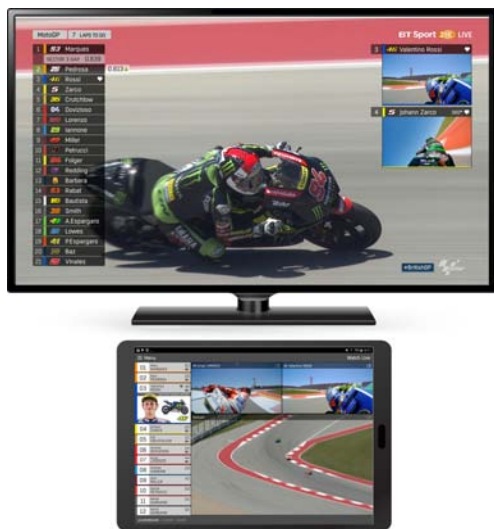
Figure 11. Advanced mode of layout design for a TV screen, where the video stream is overlaid by components with accurately specified positions (above); region mode of layout design for a tablet screen, where a screen is separated into multiple regions (below).
